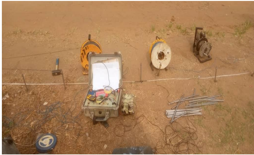
Fig. 4. Field set up for data acquisition using the VES technique. The main measuring equipment was the resistivity meter with the electrodes, cables and other accessories.
